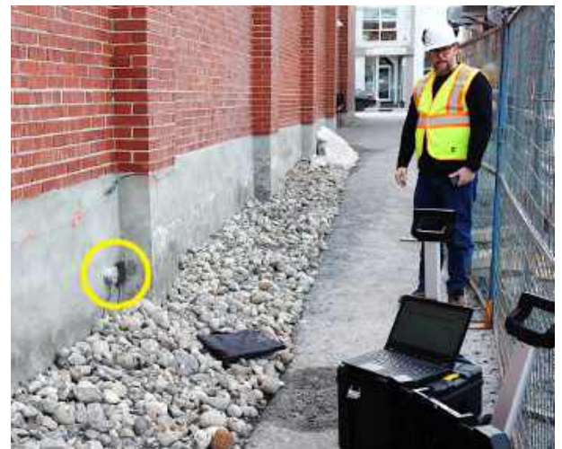
Figure 26. The MEMS and solenoid devices were mounted side-by-side along a concrete wall on an adjacent building to the construction site, 18 inches above the ground.
